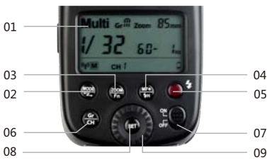
(1) LCD Panel (2) Mode Selection Button/Wireless Mode Selection (3) Zoom/Function Custom Button (4) Focus Assist Beam/High Speed Sync Button (5) Test Button/Flash Ready Indicator (6) Group/Channel Setting (7) ON/OFF switch (8) Set button (9) Select dial
