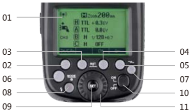
(1)LCD Panel (2)Function Button 1 (3)Function Button 2 (4)Function Button 3 (5) Function Button 4 (6) Mode selection button (7) *z Wireless Selection Button (8) Test button/Flash ready indicator (9)Set button (10) ON/OFF switch (11) Select dial
