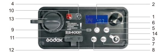
(1) Flash Output Dimmer (2) LCD Panel (3) Test Button (4) Sound Beep Outlet (5) Mode Selection Button (6) Power Switch (7) Buzz Button (8) Modeling Lamp Switch (9) Battery Level Indicator (10) Light Sensor (11) Sync Cord Jack (12) Wireless Control Port (13) Power Output Socket (14) Flash Ready Indicator
